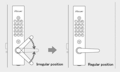
In case lever handle does not stay at correct position, it means safety device is actuated to protect from the irregular attack by force.
