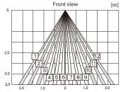
The actual detection area may become smaller depending on the ambient light, the color / material of the floor as well as the entry speed of the object.
