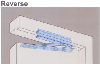
Close the door, and the door choser remains out Models and applicable standard doors Installation and Precautions of sight. Open it, and the closer's sleek lines lend beauty to your room decor. With light and smooth action, outstanding performance and superb durability, the 600U Series NHN Concealed Door Closer offers quietness and style in guest rooms, studier and other rooms.
