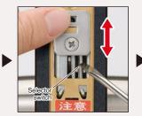
④ After operating the switch, put the holder plate back in its original position and securely tighten the screw.
